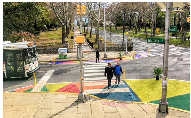
Figure 11 - Temporary Curb Bulge
